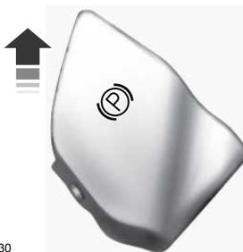
Pull the switch up to apply the electric parking brake.
