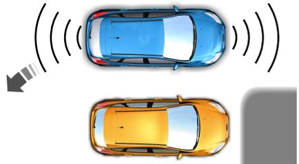
When automatic steering is finished, the touch screen displays a message and a tone sounds, indicating that the active park assist process is done. The driver is responsible for checking the parking job and making any necessary corrections before putting the transmission in Park (P).
